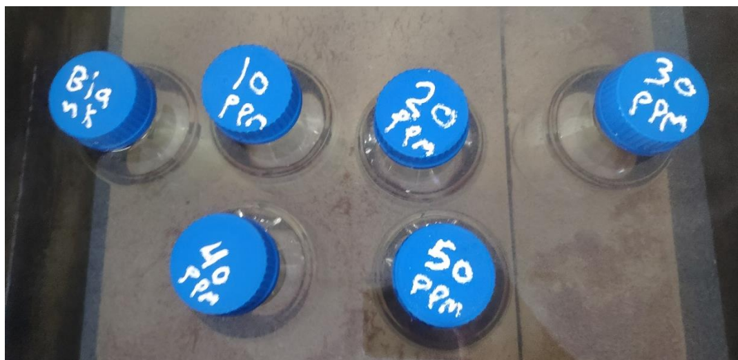
Figure 58 Place the coupons container in the water bath after injection
