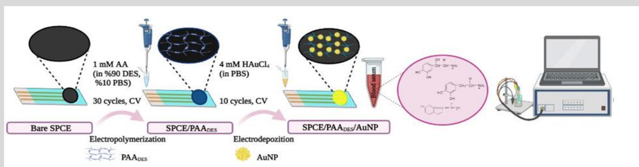
Figure 1. The preparation steps of the electrode
