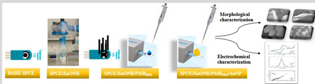
Figure 1. The preparation stage of the SPCE/ZnONR/PMB DES /AuNP sensor
