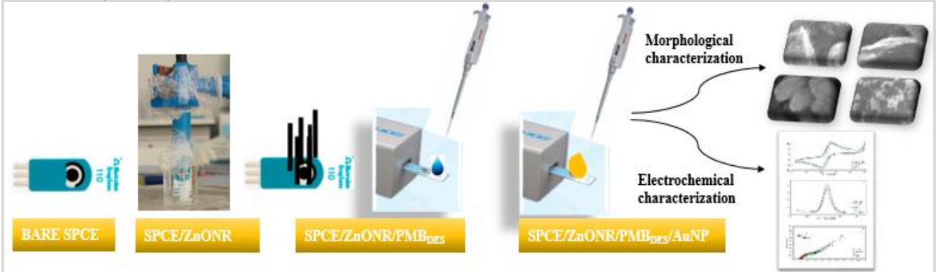
Figure 1. The preparation stage of the SPCE/ZnONR/PMB DES /AuNP sensor
