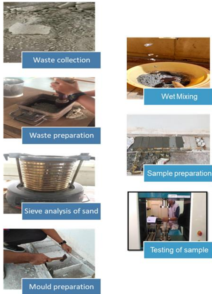
Figure 1: Experimental Study on Recycling Foundry Waste into Bricks
