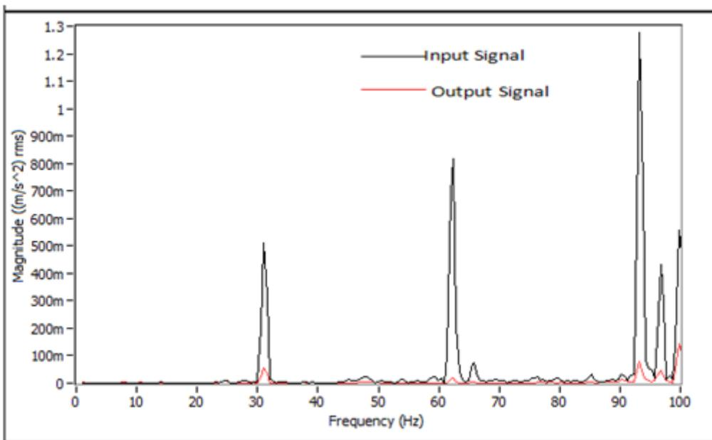
Figure 14. Frequency spectrum of the input and output signals for 10 bar recess pressure.
