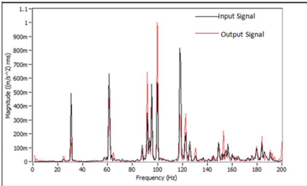
Figure 13. Frequency spectrum of the input and output signals for 8 bar recess pressure.
