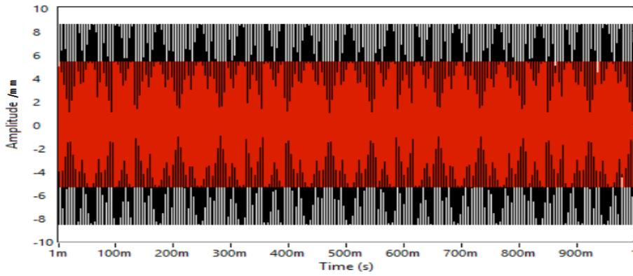
Figure 5. Time response of the input and output for 6 bar recess pressure
