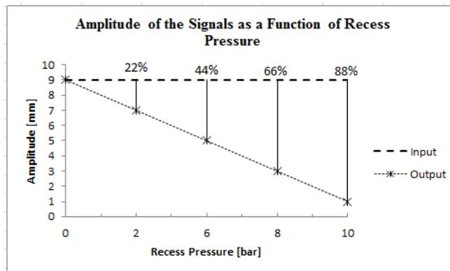
Figure 8. Percentage reduction amplitude of the Input signal when compared to the Output signal
