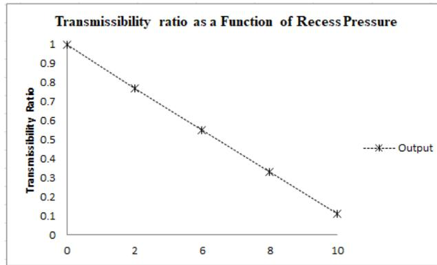
Figure 9. Transmissibility Ratio reduction against recess pressure
