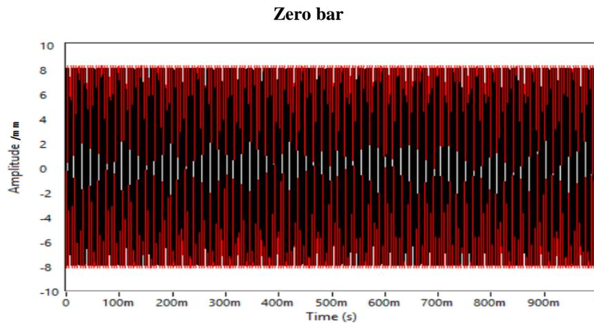
Figure 3. Time response of the input and output for 0 bar recess pressure
