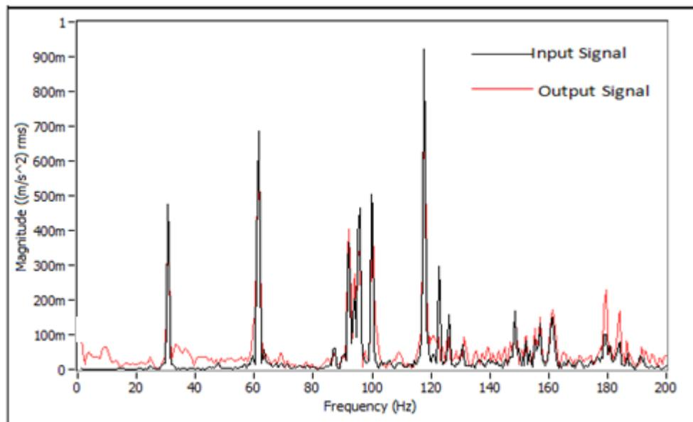
Figure 12. Frequency spectrum of the input and output signals for 6 bar recess pressure.
