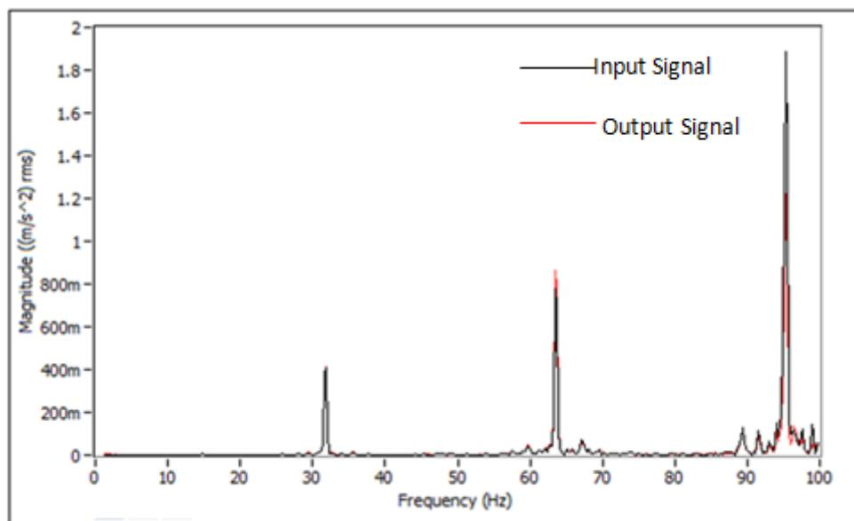
Figure 10. Frequency spectrum of the input and output signals for 0 bar recess pressure.
