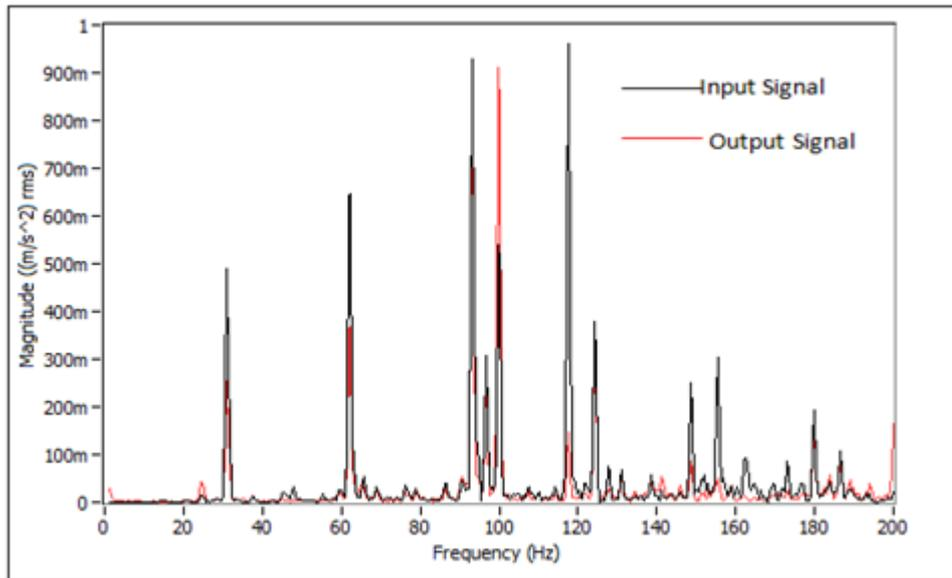
Figure 11. Frequency spectrum of the input and output signals for 2 bar recess pressure.
