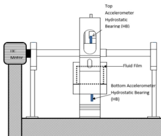
Figure 1. Experimental setup with Input Signal and Output Signal
