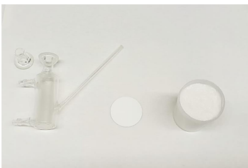
Figure 1. Franz diffusion cell and cream formulation
