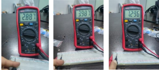
Figure 2. The difference in the value of the internal resistance for each LDR sensor, and for the same LDR sensor values used in this study (Researcher)
