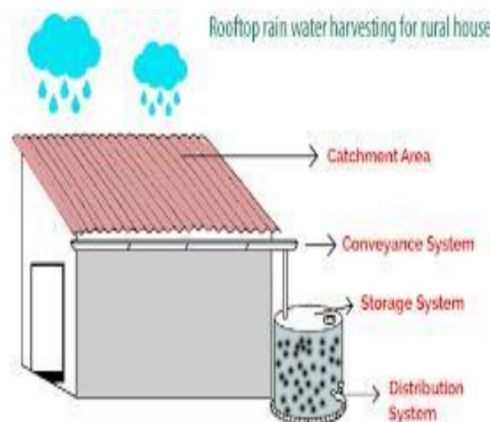
Figure 1: Rainwater harvesting system for house [2]
