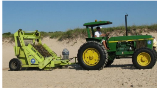
Figure 4: Hydraulic-operated beach cleaning machine
